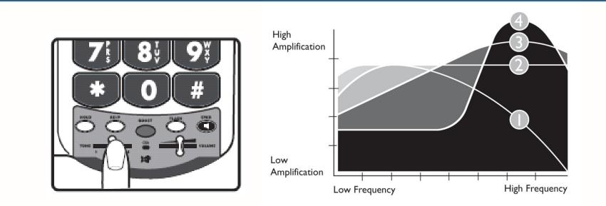
The XL45 offers four different tone settings to provide an experience that may be customized to fit a specific users need. The illustration above shows how the four settings relate to each other and the amount of amplification they give to the different frequencies of sound.
